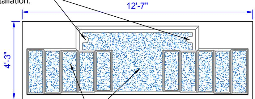
Slip resistant surface on steps and bottom of tank
