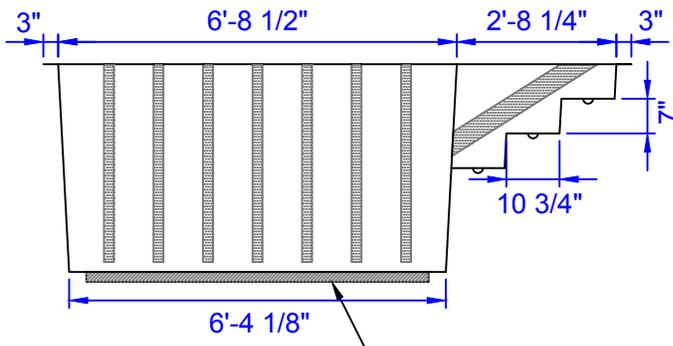
**Rear View** (4) 2x4's Molded Into Bottom Of Unit
