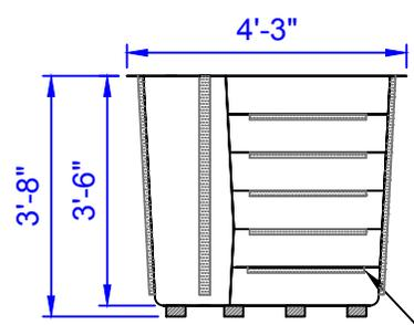
**Side View** Tubular Bracing On Sides Of Tank And Bottom Of Steps
