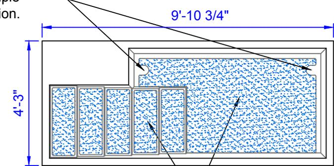
**Top View** Slip Resistant Surface on Steps and Bottom of Tank
