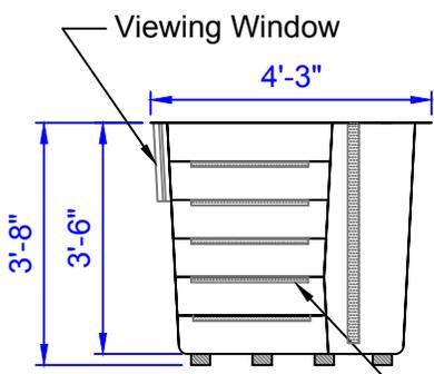
Acrylic viewing window installed by PCT
