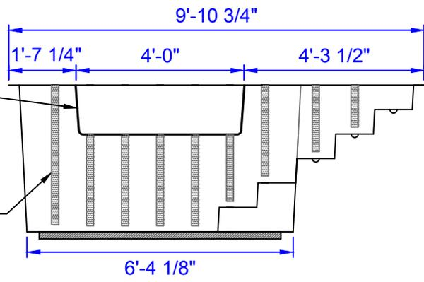
Two recessed drain locations molded into baptistery for versatile but simple installation.
