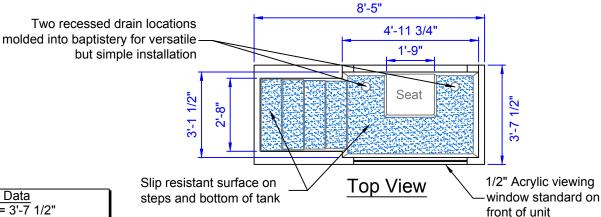
**Baptistery Data** Overall Width = 3'-7 1/2" Overall Length = 8'-5" Overall Height = 3'-6" Overall Depth = 3'-5" Unit Weight = 350 lbs. Water Capacity = 400Gallons Recommended Heater: PBH 5500 Heater System Optional Heater: PBH 11000 Heater System Available Colors Blue White Aqua Beige Note: Color samples available at customers request
